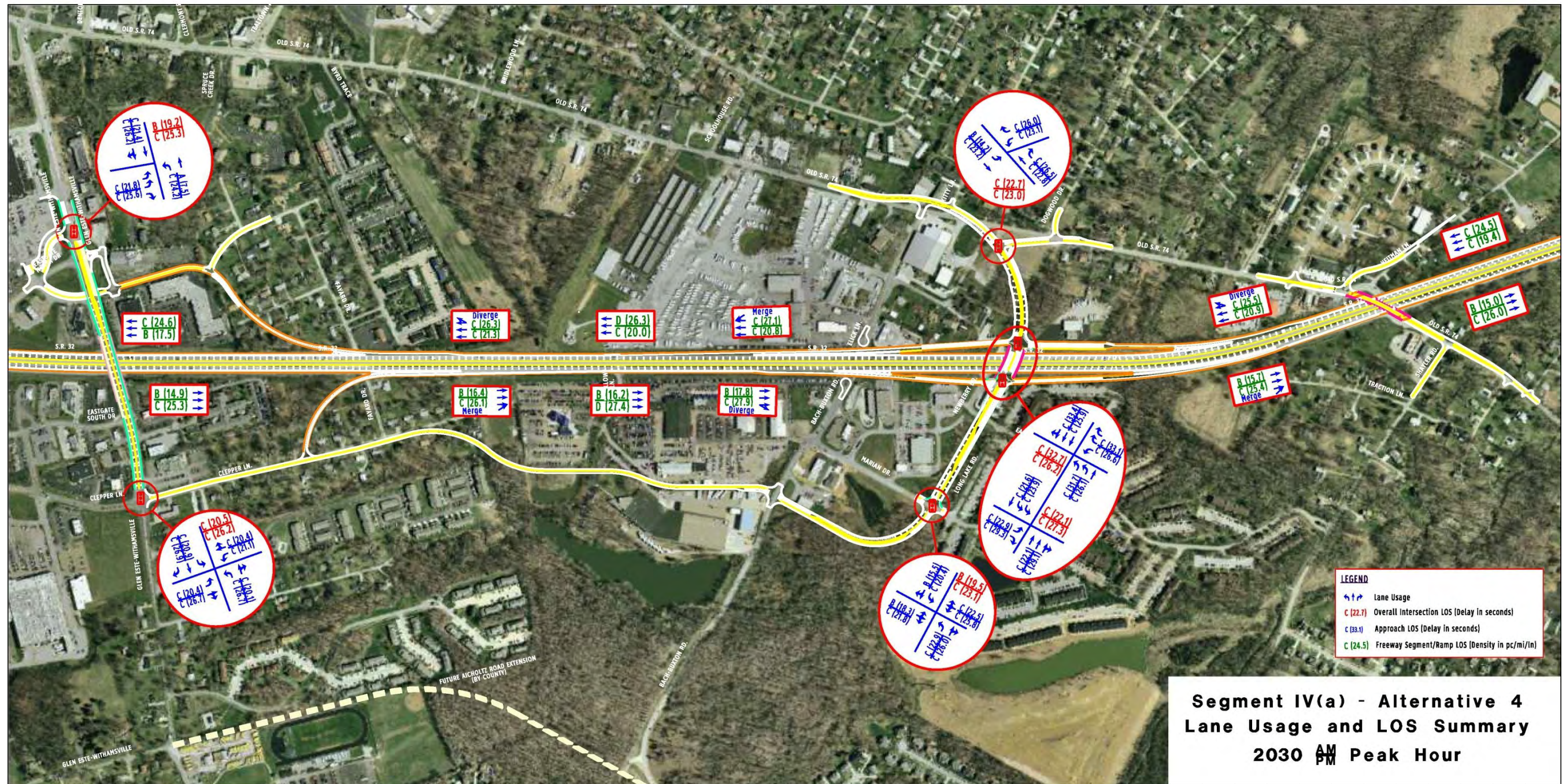
Figure 11: Alternative 4 (with Glen Este ramps) Capacity Analysis
